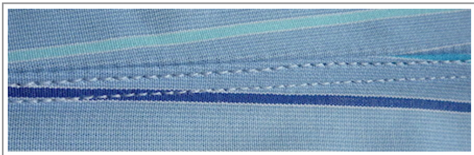
Single-needle stitching: inside and outside looks
